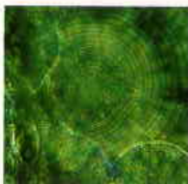
Figure 2. Spherulitic chalcidony in polycrystalline aggregates. Specimen from Cottonwood Springs Basalt, Cathedral Mountain Quadrangle, west Texas. X360.
