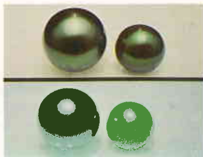
Figure 11. Green-black pearls. Left: cultured black pearl. Right: silver treated. Conventional color image (above) and infrared image (below).
