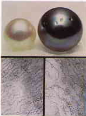
Figure 3. Microscopic observation of stripe patterns of Akoya pearl (left) and cultured black pearl (right) (60x).
