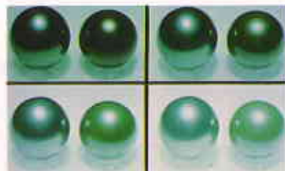
Figure 15. Images of infrared color film with varying exposures. Above left: optimum exposure. Above right: one scale in excess of the optimum exposure. Below left: three scales in excess. Below right: five scales in excess. The cultured black pearl (to the left of all four pictures) is clearly distinguished from the silver salt treated pearl (to the right of all four pictures).
